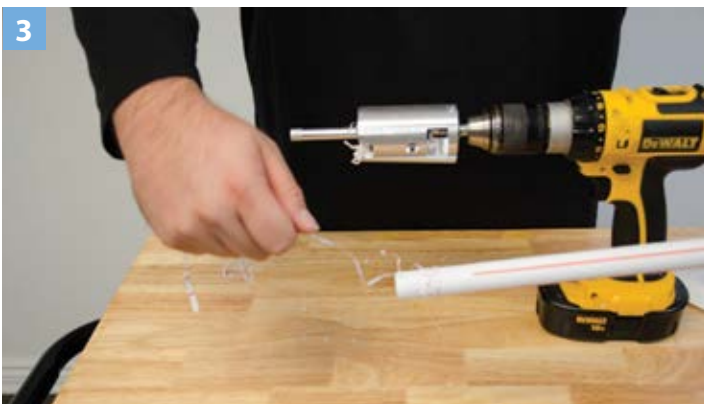
3) Remove any burrs from the pipe end ensuring you do not touch the pipe end with your hands as oils on the skin can lead to a faulty weld.
