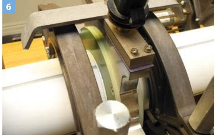
6) Once the bead has reached the correct height, the pressure should be decreased to the heating + drag pressure. The heating pressure can be found in table 44. Hold the heating pressure for the duration of time shown in table 39 on page 62. Note: Some machines lock into
