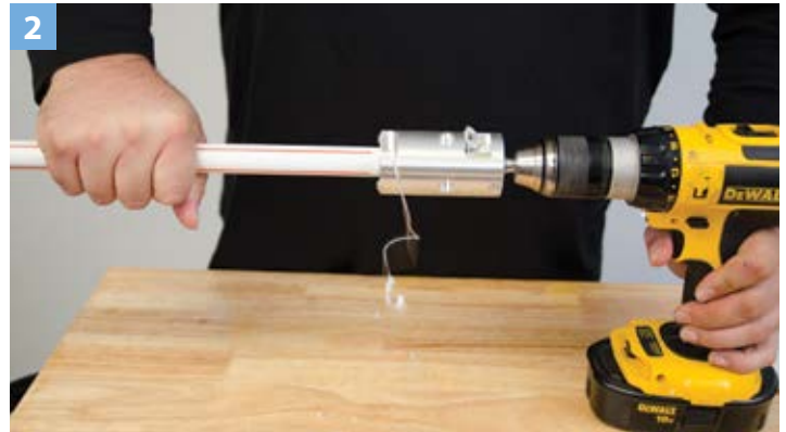
2) Cut pipes square and scrape the pipe ends to ensure they are free from contaminants. Note: Special scraping tools designed to aid in this procedure are available however, as an alternative a paint scraper can be used as well.
