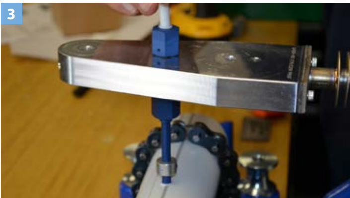
3) Weld the pipe and the plug at the same time, being careful not to create internal burrs.
