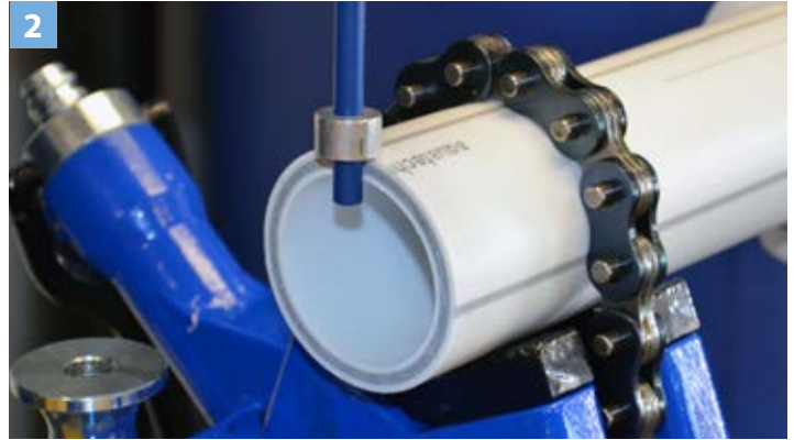
2) Adjust the depth gauge on the repair die to just past the thickness of the wall. The thickness of the wall can be found in the aquatechnik ® Piping Solutions section of this manual.
