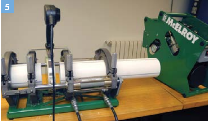
5) Attach the heating plate to the butt fusion machine and apply the combined pressure (drag + welding pressure) until a bead is present. The bead should be 1/32" (1 mm) for 6-8" diameter pipe and 1/16" (1.5mm) for 10" diameter pipe.
